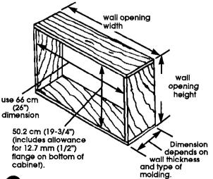
**4** Insert the frame in the wall opening. Square the level frame. Nail frame securely to the wall studs.
